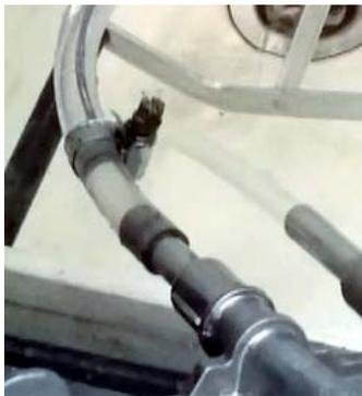
**Fig. 2:** The hose inlet facilitates the coring of long channels.
